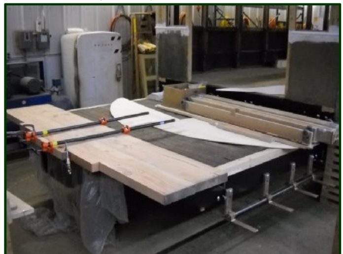
Here's one of the end platforms. Note the templates used to trace the curve on the end of the platform to help making the proper cut.
