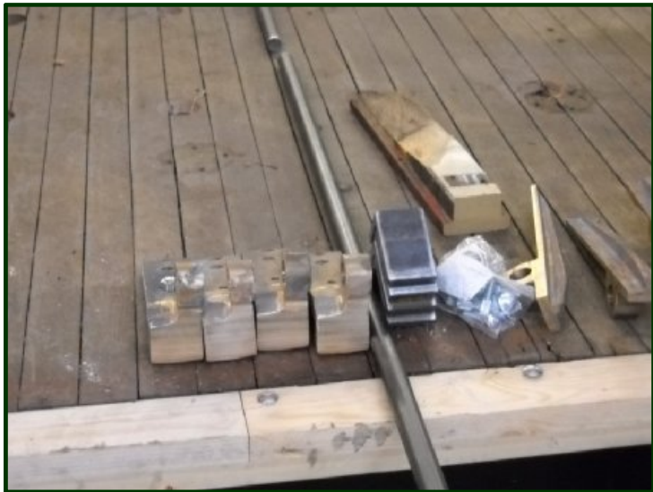
Here's just a few of the over 150 parts that'll make up the folding step and door mechanism. The mechanism will be built from scratch following the original St. Louis Car Company plans we obtained several years ago.
