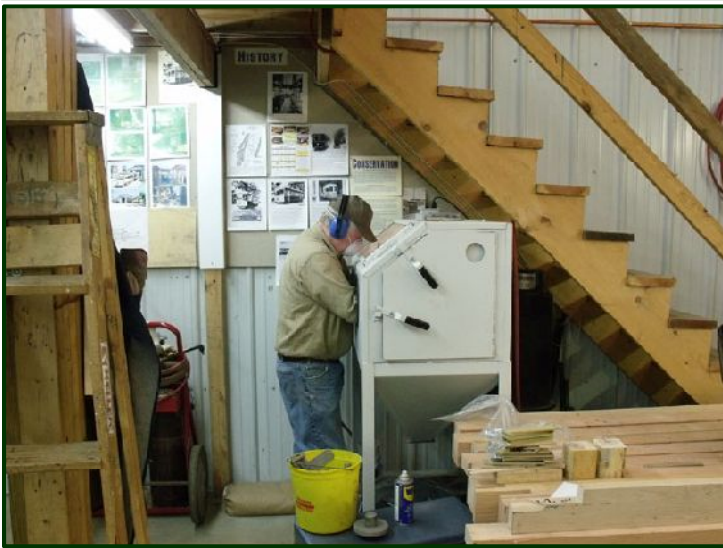
Dick Zawacki is seen here sand-blasting some metal parts for Winona No. 10.
